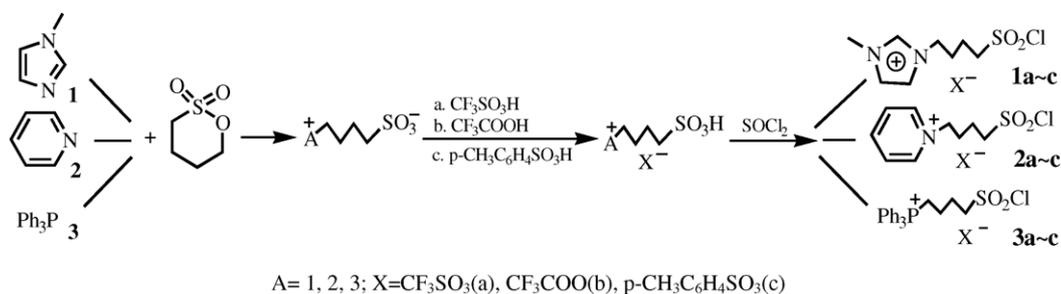
Scheme 2. Synthesis of sulfonyl chloride functionalized ionic materials.
