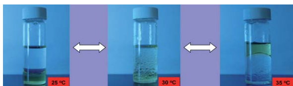
Fig. 2 Reversible phase reversion of a [AC 8 Im]DCA/H 2 O mixture as the temperature varies.
