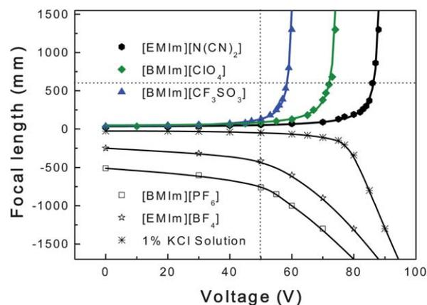
**Fig. 3** Change of focal length of five typical ILs and saline-based EVFLL with applied voltage. The solid lines are theoretical curves.
