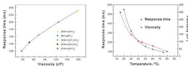
**Fig. 5** Response times of five IL-based EVFLL with different viscosities (left) and [EMIm][ClO<sub>4</sub>]-based EVFLL at variable temperature (right).
