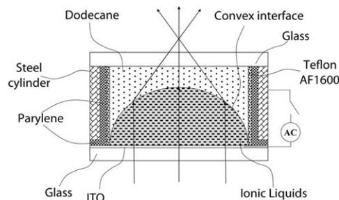
**Fig. 1** Schematic cross section of an IL-based EVFLL.
