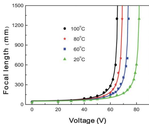
**Fig. 4** Change of focal length of EMImClO<sub>4</sub>-based EVFLL with applied voltage at variable temperature. The solid lines are theoretical curves.
