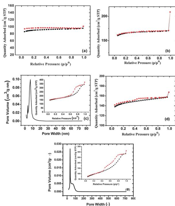
**Fig. 1** N<sub>2</sub> adsorption–desorption isotherms of (a) RF-no IL, (b) RF-2.5%BMImBF<sub>4</sub>, (c) RF-10%BMImBF<sub>4</sub>, (d) RF-15%BMImBF<sub>4</sub> and (e) RF-10%BMImBF<sub>4</sub> (before carbonization but removing ionic liquid) and BJH pore distributions of (c) and (e).
