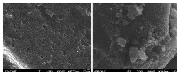
**Fig. 2** SEM pictures of RF-no IL (left) and RF-10%BMImBF<sub>4</sub> (right).
