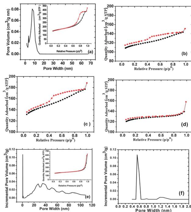
**Fig. 3** N<sub>2</sub> adsorption–desorption isotherm of (a) RF-10%OMImBF<sub>4</sub>, (b) RF-10%EMImBF<sub>4</sub>, (c) RF-10%BMImPF<sub>6</sub>, (d) RF-10%BMImN(CN)<sub>2</sub> and (e) RF-10%BMImCl; BJH pore distribution of (a) RF-10% OMImBF<sub>4</sub>; DFT pore distribution of (e) RF-10%BMImCl and enlarged DFT pore distribution of (f) RF-10%BMImCl in the range of 0–2 nm.
