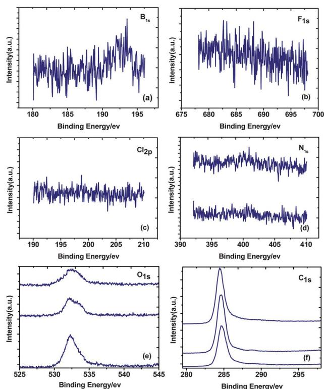
**Fig. 5** XPS spectra of (a) B<sub>1s</sub> of RF-10%BMImBF<sub>4</sub>, (b) F<sub>1s</sub> of RF-10%BMImBF<sub>4</sub>, (c) Cl<sub>2p</sub> of RF-10%BMImCl, (d) N<sub>1s</sub> of RF-10%BMImBF<sub>4</sub> (top) and RF-10%BMImCl (bottom), (e) O<sub>1s</sub> of RF-10%BMImBF<sub>4</sub> (top), RF-10%BMImCl (centre) and RF-no IL (bottom) and (f) C<sub>1s</sub> of RF-10%BMImBF<sub>4</sub> (top), RF-10%BMImCl (centre) and RF-no IL (bottom).
