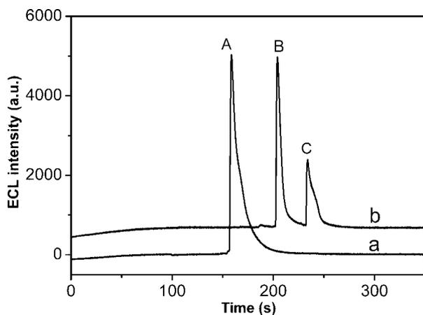
**Figure 3.** Electropherograms of mixtures of 2  $\mu$ M TPA and 5  $\mu$ M DBAE when (a) 10 mM PBS and (b) 10 mM BDS were used as running buffers, respectively. ECL intensities of (A) unseparated of TPA and DBAE, (B) TPA, (C) DBAE. Conditions are the same as in Fig. 1.
