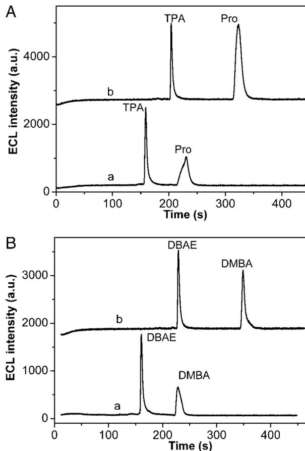
**Figure 1.** Comparison results of CE with ECL detection using (a) 10 mM PBS (pH 7.4) and (b) 10 mM BDS as running buffers. Mixtures of (A) 0.2  $\mu\text{M}$  TPA and 50  $\mu\text{M}$  Pro and (B) 2  $\mu\text{M}$  DBAE and 10  $\mu\text{M}$  DMBA. Conditions: detection potential, 1.2 V; 5 mM  $\text{Ru}(\text{bpy})_3^{2+}$  with 50 mM PBS (pH 7.4) in the detection reservoir; electrokinetic injection, 8 s at 12.5 kV; separation voltage, 15 kV.
