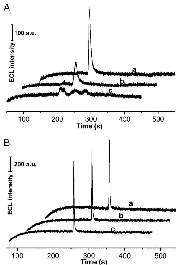
**Figure 4.** Different effects of (A) 10 mM SDS or (B) 10 mM BDS used as additives in 10 mM PBS running buffer on the repeatability of ECL intensity of TPA by CE with ECL detection. (a–c) Electropherograms of 0.1  $\mu\text{M}$  TPA, which was injected consecutively three times, respectively. Conditions are the same as in Fig. 1.
